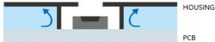
Figure 2: The sensor is completely isolated from the dead zone air inside the housing, which minimizes the influence of the airtight air inside the housing on the sensor
